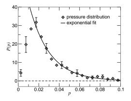
FIG. 14: Pressure distribution on the contact region between two elastic bodies with realistic interfaces. The linear lines show the exponential decay (tails) of each distribution.
