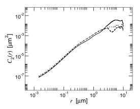
FIG. 13: Height-difference correlation function in a 2D plane for three different slices of a realistic surface. The values of the parameters in the corresponding self-affine model are: H = 0.84,  $q_{\rm s} = 2\pi \, 10^{-3}/a$ .
