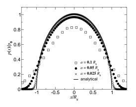
FIG. 11: Normalized pressure profile of a one-dimensional Hertzian contact using the exponential wall interactions with a screening length of  $\sigma = 0.25 \cdot a$ . Different degrees of discretization of the elastic manifold were used. The radius of curvature of the parabolic tip was chosen to be  $128 \cdot a$ , which corresponds to roughly 40 nm if a is a typical interatomic distance of 3 Å. The contact radius  $R_c$  was varied by applying different loads.
