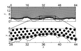
FIG. 5: Comparison of the contact formation of a manifold with a rough substrate: Small, full circles show atomic positions of atoms in the full MD, while large, open circles represent the degrees of freedom used in the GFMD simulations. The lower graph is a magnification of a part of the upper graph.
