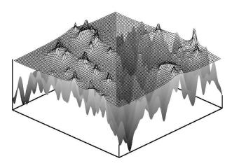
FIG. 8: Illustration of a GFMD configuration representing a three-dimensional, semi-infinite, elastic solid that is pressed against a rigid, self-affine, fractal substrate. The right half of the Green's function layer is represented in a more transparent fashion that the left half. The direction normal to the interface is enlarged with respect to the in-plane directions.
