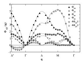
FIG. 1: Dispersion of the surface stiffness coefficients for a semi-infinite (111) surface of an fcc lattice. Some components of the  $\Phi_{\alpha\beta}(\mathbf{q})$  matrix are multiplied by a factor of four for reasons of optical resolution. The lines correspond to fits whose adjustable parameters are given in Section III.
