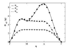
FIG. 6: Numerical (symbols) and analytical<sup>17</sup> (lines) results for the diagonal elements of  $\Phi_{\alpha\beta}(\mathbf{q})$  in the simple cubic crystal lattice along lines connecting high symmetry points in the Brillouin zone.
