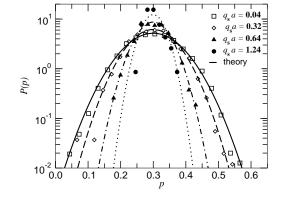
FIG. 12: Pressure distribution for different magnifications at the interface of a rough interface in complete contact with an elastic solid. The distribution is centered at the nominal contact pressure. Full and broken lines are based on a parameter-free theory by Yang et al. [8].
