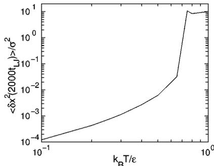
FIG. 5. Mean-squared displacement of top wall along a single coordinate,  $\langle \delta x^2(t) \rangle$ , after time  $t=2000t_{LJ}$  as a function of  $T$  at  $f_z = 0.75\epsilon/\sigma$ . The walls are commensurate and  $N=32 \times 32$ .
