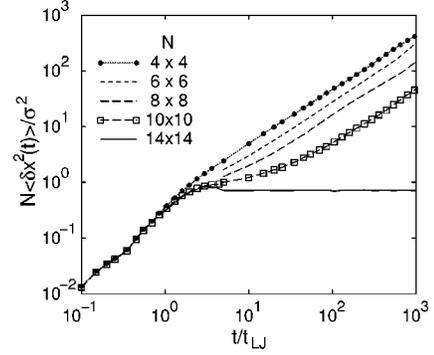
FIG. 1. Mean-squared displacement of top wall along a single coordinate,  $\langle \delta x^2(t) \rangle$ , as a function of time  $t$  for commensurate walls of the indicated sizes. Displacements are multiplied by  $N$  to remove the trivial dependence on wall mass. Here  $f_z = 1.2\epsilon/\sigma$  and  $k_B T = 0.8\epsilon$ .
