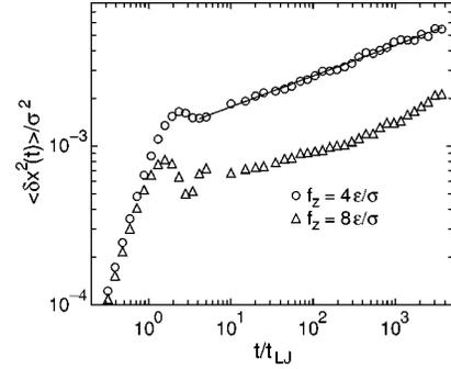
FIG. 8. Mean-squared displacement of top wall along a single coordinate,  $\langle \delta x^2(t) \rangle$ , as a function of time  $t$  for two different normal forces and  $k_B T = 0.8\epsilon$ . Bottom and top wall are incommensurate and  $N = 31 \times 36$ . The straight line is a fit to a power law  $t^\alpha$  with  $\alpha = 0.194 \pm 0.004$ .
