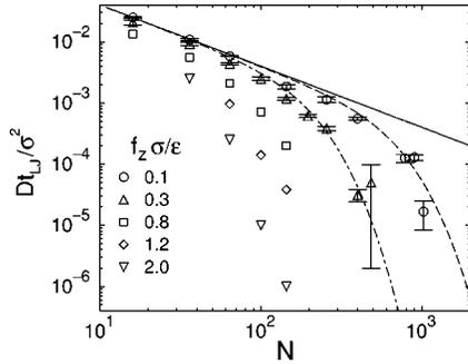
FIG. 2. Diffusion constant calculated from the time to move by  $\sigma$  as a function of the number of atoms per wall  $N$  at the indicated values of  $f_z \sigma / \epsilon$  and  $k_B T = 0.8 \epsilon$ . A solid line shows the free diffusion constant  $D_0$ . Dashed and dot-dashed lines show fits to Eq. (3.3) for  $f_z = 0.1$  and  $0.3 \epsilon / \sigma$ , respectively.
