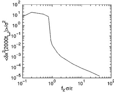
FIG. 4. Mean-squared displacement of top wall along a single coordinate,  $\langle \delta x^2(t) \rangle$ , after time  $t=2000t_{LJ}$  as a function of  $f_z$  at  $k_B T=0.8\epsilon$ . The walls are commensurate and  $N=32 \times 32$ .
