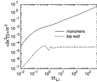
FIG. 3. Mean-squared displacement along a single coordinate,  $\langle \delta x^2(t) \rangle$ , of individual monomers and of top wall as a function of time  $t$  at  $f_z = 10 \epsilon / \sigma$  and  $k_B T = 0.8 \epsilon$ . The walls are commensurate and  $N = 32 \times 32$ .
