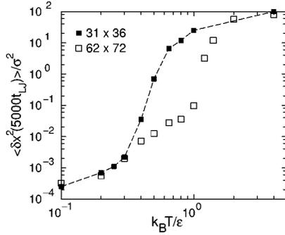
FIG. 10. Mean-squared displacement of top wall along a single coordinate,  $\langle \delta x^2(t) \rangle$ , after time  $t = 5000 t_{LJ}$  as a function of temperature for two different system sizes at  $f_z = 2\epsilon/\sigma$ . The results for the larger wall were multiplied by a factor of four to remove the trivial dependence on wall mass.
