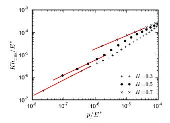
FIG. 2: (Color online) Dimensionless interfacial stiffness  $Kh_{\rm rms}/E^*$  as a function of pressure  $p/E^*$  in the finite-size region for  $L/\lambda_1=4096$  and different Hurst exponents H. All calculations are for  $L/\lambda_r=1$ . Solid lines show a fit to the first four data points.
