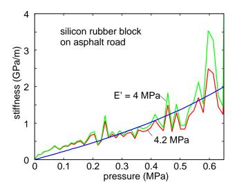
FIG. 6: (Color online) The normal contact stiffness as a function of the applied nominal contact pressure for a silicon rubber block (cylinder shape with diameter D=3 cm and height d=1 cm) squeezed against a road asphalt surface. The green and red lines are obtained from the measured p(s) relation using (7) with E'=4.0 MPa and 4.2 MPa (see text) while the blue line is the theory prediction.
