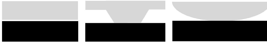
Figure 8: Schematic representation of initial geometries. Left: Flat surfaces. Middle: Blunt tip on substrate. Right: Curved tip on substrate.
